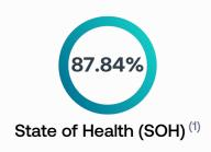
Remaining usable capacity / Usable capacity when new (2)
