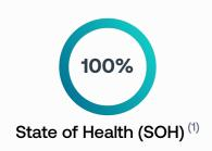
Remaining usable capacity / Usable capacity when new (2)
