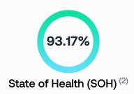
Remaining usable capacity / Usable capacity when new (3)
